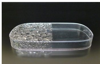
Right side of the plastic container is coated with the new coating showing no beading of water
